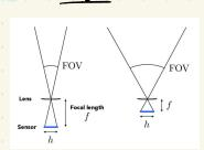
smaller focal length -> LARGER FOV larger focal length -> SMALLER FOV Smaller sensor Size -> smaller FOV
